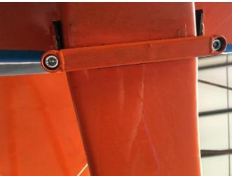
Production tolerances mean that in very rare cases 4 washers may be needed on one side of the clamp bracket – the SB pack contains 7 washers in case. However, the aircraft fitted to date did not show this requirement.
