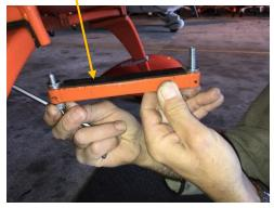
3. Trim the top fuselage rubber so that it is flush with bracket end as shown, so rubber does not foul new washer. Also ensure the top rubber is evenly and centrally positioned around the leg. Contact EuroFOX Aviation if you need new rubbers
