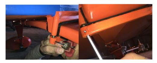
2. Check the top and bottom U/C rubbers are not split or deformed due to excessive prior clamping for example. Check the lower rubber is still adhered to the clamp bracket and not the u/c leg as shown (left below). If the lower rubber has lost its adhesion to the clamp bracket, apply contact adhesive to refix (right below).
