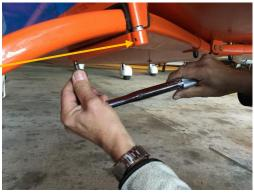
7. Determine where the M8 bolt split pin locating hole is in relation to the clamp bracket split pin locating hole and readjust the bolt torque to line them up. Then insert the securing split pin. Depending where these locating holes line up for the split pin, you will need to add a little more torque (max 24Nm), or slacken off the bolt to insert the split pin. DO NOT overtighten the bolt more than 24Nm. If this is needed to line up the split pin holes, slacken off the bolt torque in preference.
