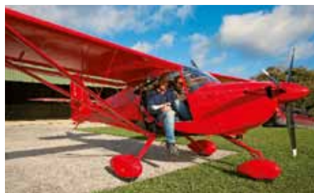
Gas strut holds the top hinged door well clear up under the wing, making for an easy entry and exit which is unhindered by the main gear
