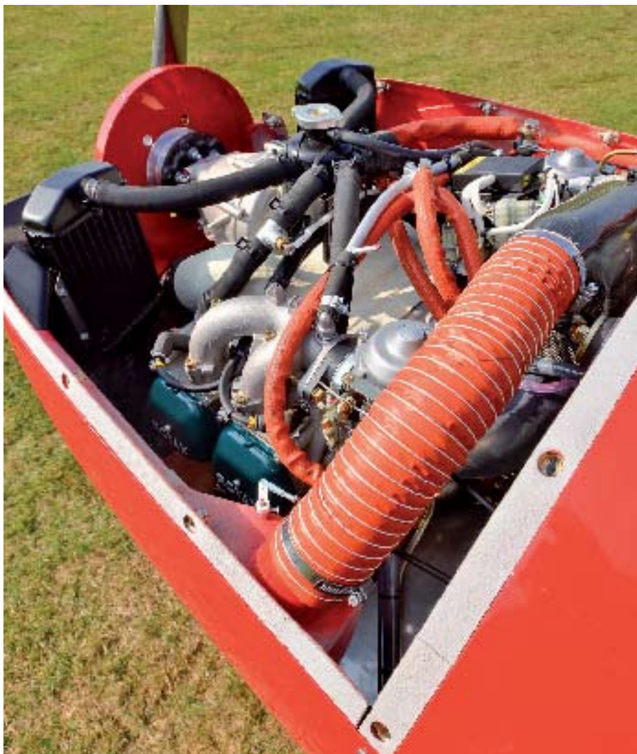
Good to see a quickly detachable cowling for the typically busy Rotax 912 engine installation
